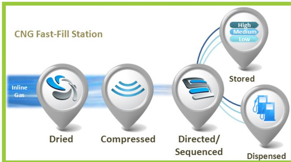
Cascade fast-fill stations primarily fill from storage tanks and are typically used for retail applications or vehicles that require refueling at varying times. Some fleet operations and most public CNG stations are examples of a cascade fast-fill configuration.
