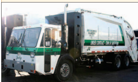
This Crane Carrier truck is one of 23 CNG powered trucks purchased by contract haulers in response to the Town of Smithtown's (NY) natural gas truck requirement.
