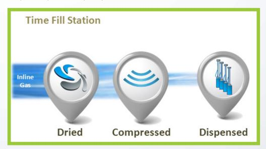
Fleets of vehicles that return to central locations for periods of time frequently utilize the time-fill configuration. This is a lower cost option and is a preferred method of refueling refuse trucks, school buses and other fleets with similar refueling requirements. Time-fill stations have significantly lower equipment and installation costs because they do not require storage, priority, or sequential refueling components.
