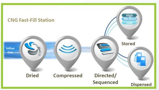
Cascade fast-fill stations primarily fill from storage tanks and are typically used for retail applications or vehicles that require refueling at varying times. Some fleet operations and most public CNG stations are examples of a cascade fast-fill configuration.
