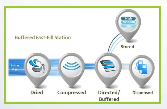
Buffer fast-fill stations are ideal for high fuel use vehicles that require immediate refueling, one after another. Taxis and transit buses frequently utilize this configuration due to their need to sequentially refuel and also because of the overall fuel demand of these types of vehicles. Buffer systems primarily fuel directly from the compressor into the vehicle and therefore require a smaller quantity of storage.
